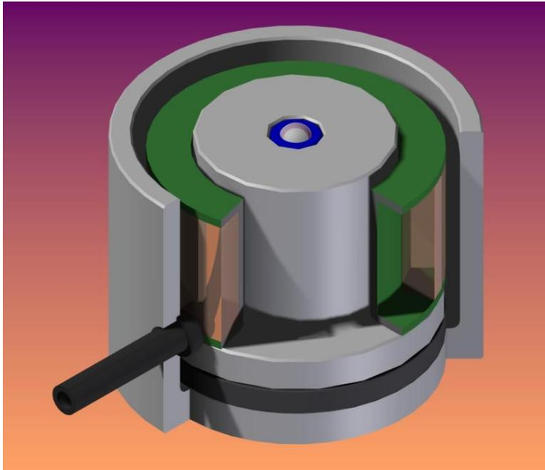
HMER devices incorporate a permanent magnet so that high holding force is developed to a flat ferromagnetic component without external power being applied. Power is applied to the device with reverse polarity to counter the field due to the permanent magnet and release the 'keeper' component.
