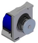
**Spring** - Addition of a return spring is a common modification, these can be fitted in many different ways either externally or internally. External springs can be secured with a staked disc, springs can also be secured with an e-ring, shoulder machined on plunger, or fitted in a groove machined in plunger. Conical springs can have shorter compressed length, and help prevent end of the
