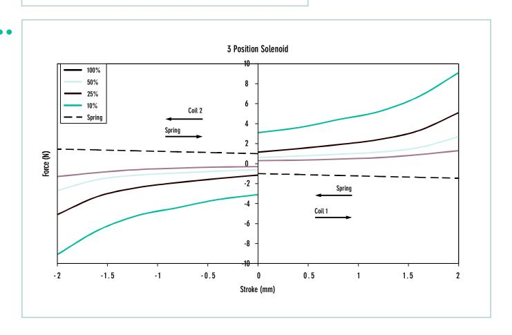
The 3-position solenoid can be produced in open-frame construction, or in tubular construction. Three different spring options are offered for most types. Option A is standard and will work with any duty cycle. Options B and C have stronger springs and will generally only work at intermittent duty cycle, refer to graphs for details.
