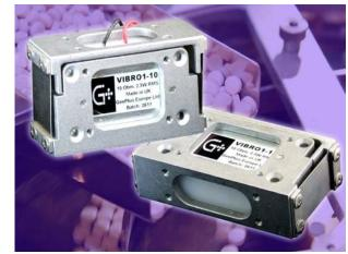
smaller the vibratory movement. Because the VIBR01 is actuated by the application of energy to rare earth magnets, unlike the more commonly used motorised assemblies, it has no sliding parts so is not subject to wear or mechanical faults.
